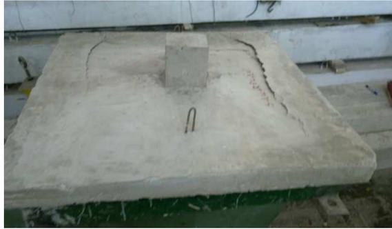
Tested slab with RPC ( $V_f$  2%) in critical zone (S5)
