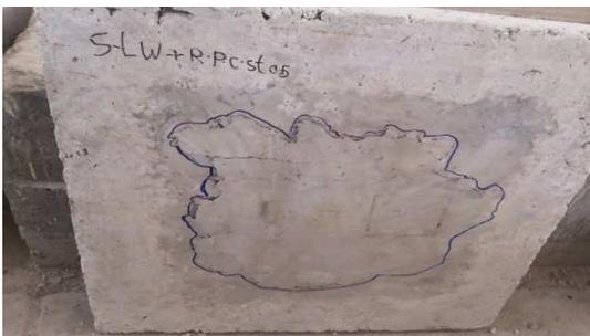
Tested slab with RPC ( $V_f$  0.5%) in critical zone (S3)
