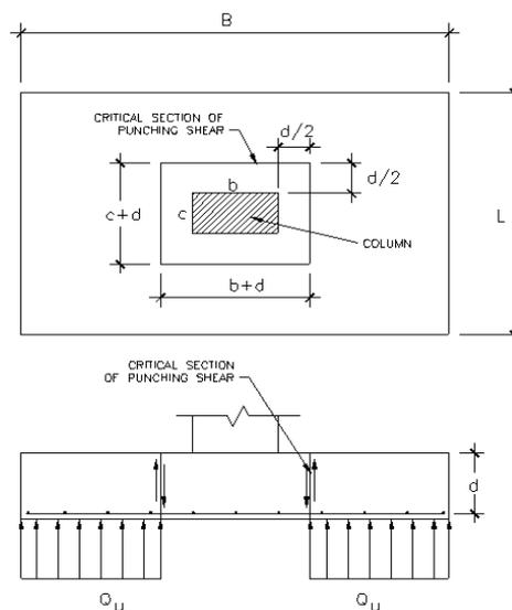
Figure (1): Critical Sections of Punching Shear [2]
