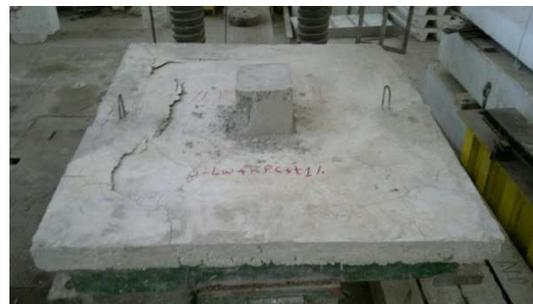
Tested slab with RPC ( $V_f$  1%) in critical zone (S4)
