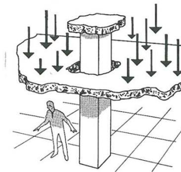
Plate 1: Punching Shear Failure [2]
