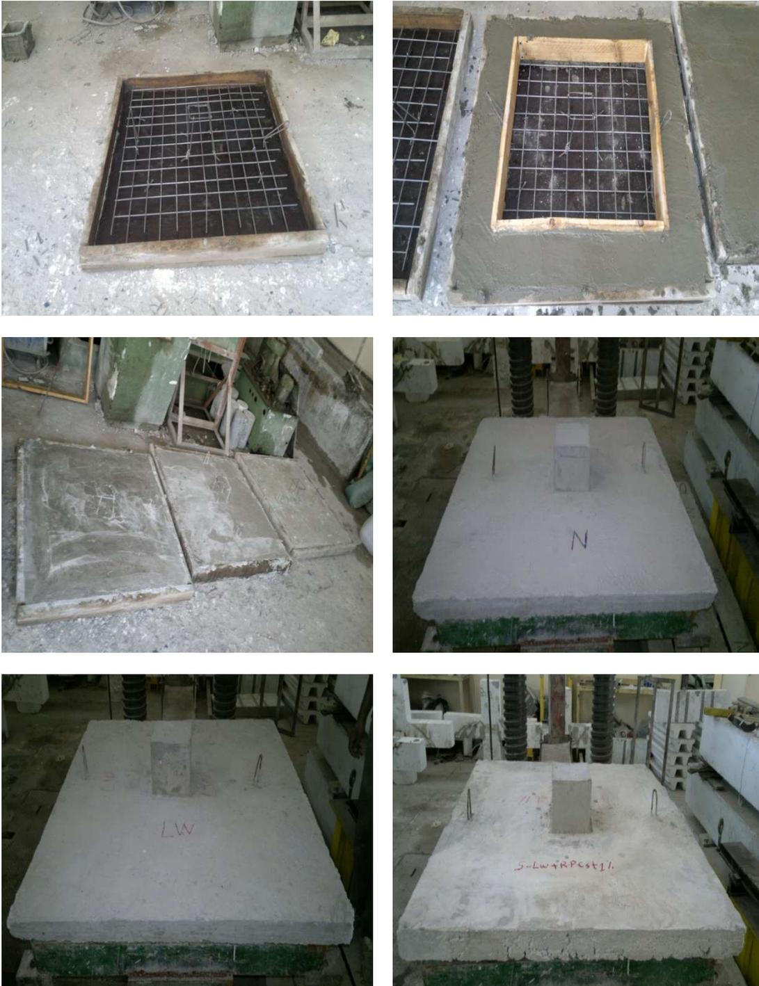
Plate 3: Molds, Reinforcements and Tested Slabs
