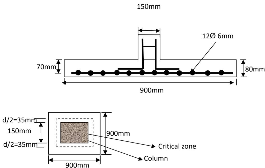
Figure 2: Dimensions of the tested slabs
